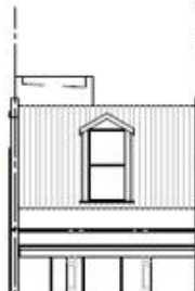
Later dormer additions removed, with smaller, more traditional dormers installed
